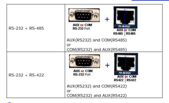
You cannot make use of AUX (RS232) port and AUX (RS485, 422) part at the same time. Also it is not available to use of COM (RS232) port and COM (RS485, 422) part together.
